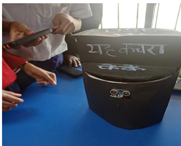
Image 41: Student-made smart dustbin with sensor-based lid
