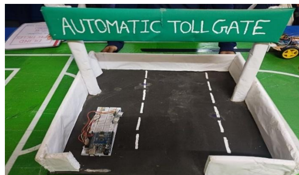
Image 40: Automatic Toll Gate - a student-built prototype using sensors and electronics
