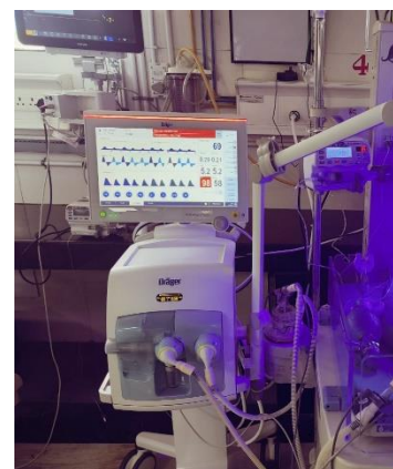
Figure 48: Neonatal Ventilator with HFO
