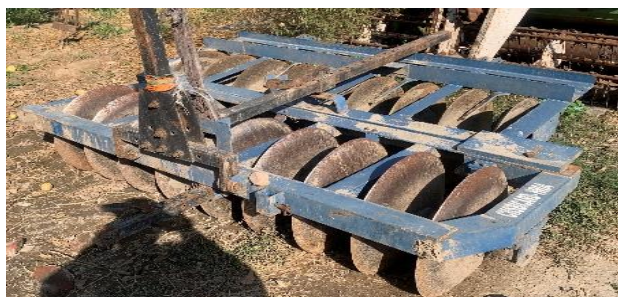
Harrow (Breaks up & smoothen soil bed)
