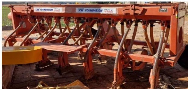
Happy Seeder (Manages residue through incorporation)
