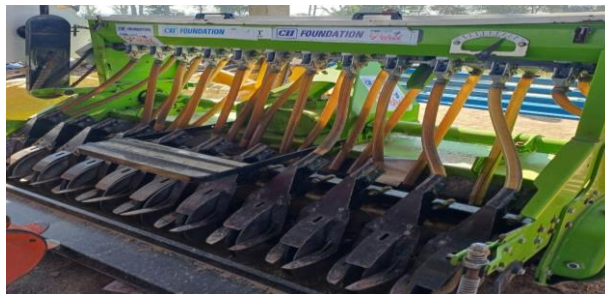
Super Seeder (Mix stubble in soil, prepare land & sow)
