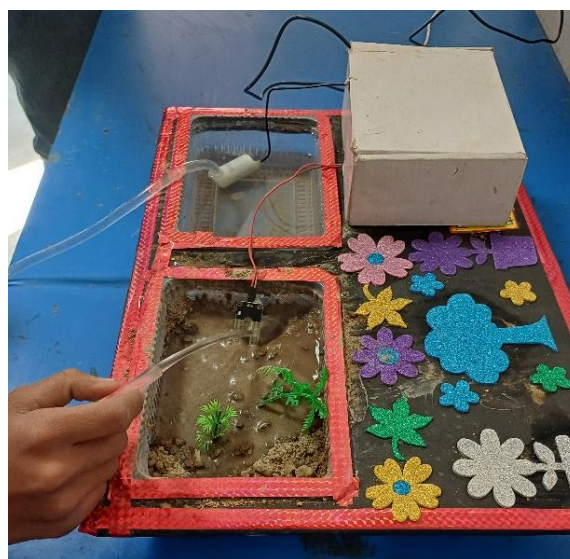
Figure 70: Establishment of Tinkering Lab - Soil Moisture Detector
